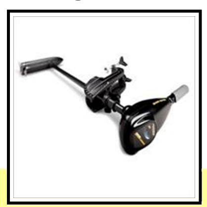
**Description**: MinnKota's Endura C2 45 is designed to offer durability, reliability and power in an affordable package. Features 45 lbs. of thrust on a 12 volt battery (battery not included). 5 forward speeds & 3 reverse, standard shaft length of 36". Telescoping handle extends to 6". Also features lever lock bracket and indestructible composite shaft.
